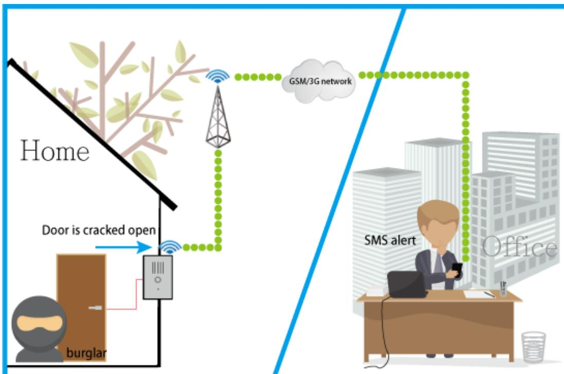
2. When the door is cracked open by a burglar, the GSM intercom will notify the user by SMS alert.
